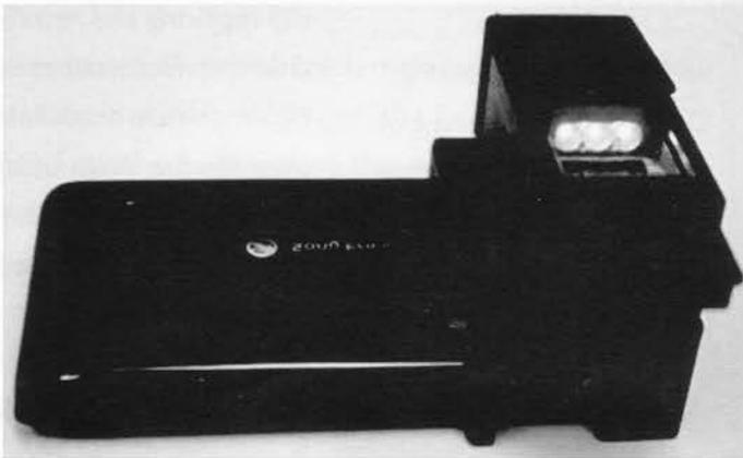
Fig 1.2. Ozcan's fluorescent microscope attached to a Sony Ericsson mobile phone.
