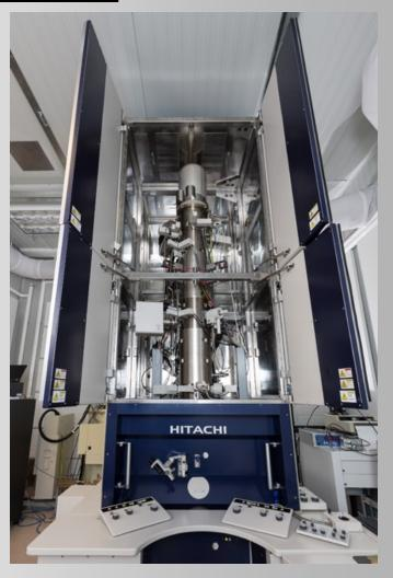
The HF-3300V scanning transmission electron holography microscope (STEHM) is now in operation at the University of Victoria. It is capable of resolving atoms at 40 picometers. That is an order of magnitude better than a standard electron microscope.
