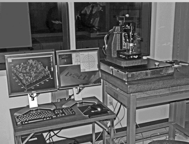
Ambios Q AFM on vibration dampening table and platform
